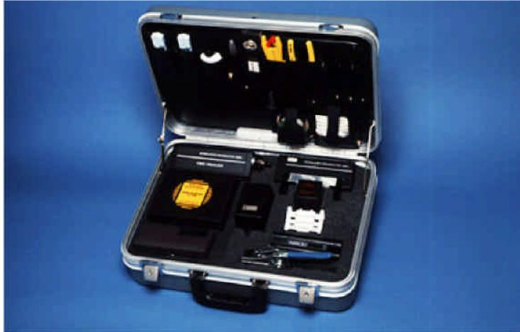
The NSK-12 is a complete tool kit designed for installing and maintaining a fiber optic network. This kit includes the Norland Fiber Visualizer with all the fiber preparation and splicing tools necessary to make a mechanical splice.
