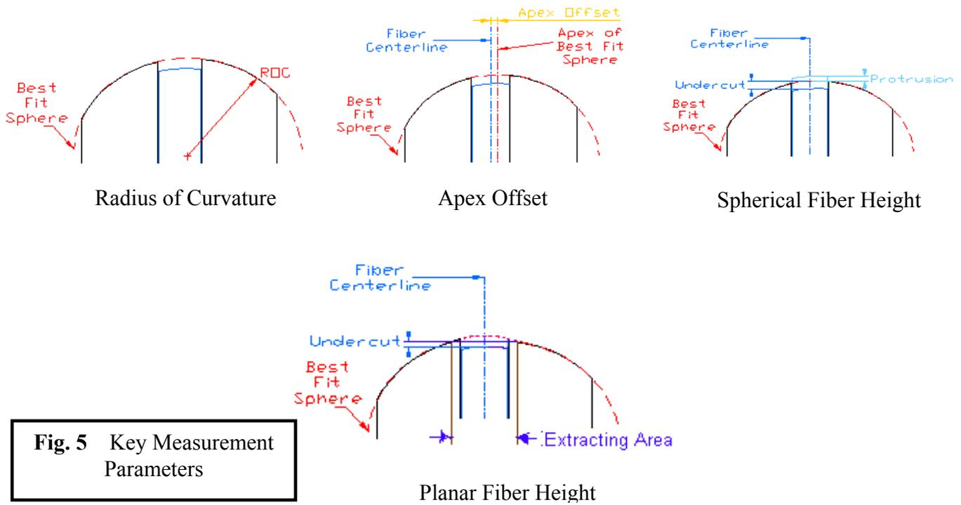
**Fig. 5** Key Measurement Parameters
