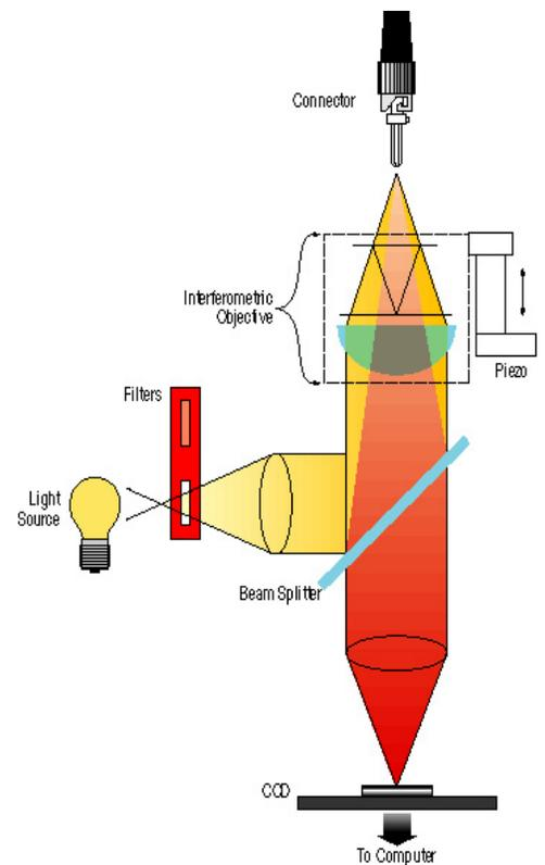
**Fig. 1** Optical Path for Interferometer
