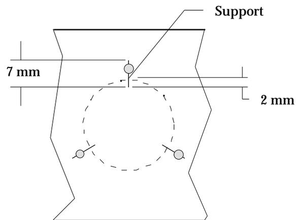
Figure 2. Placement of the temporary supports.
