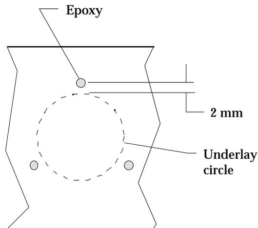
Figure 1. Placement of the epoxy points.
