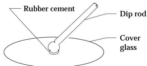
Figure 4. Picking up the cover glass
