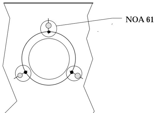
Figure 7. Starting to flow the NOA 61 under the cover glass.
