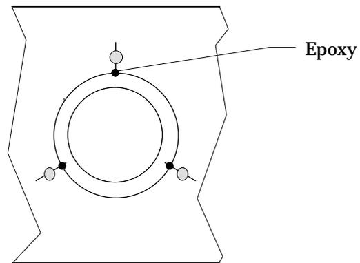
Figure 6. Epoxy points in place
