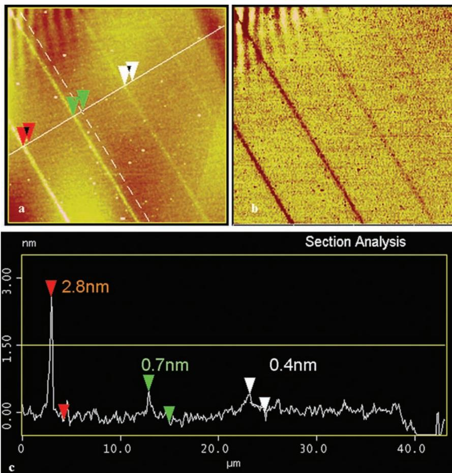
**Fig. 3.** Lines produced at increasing scanning speeds, yielding structures with decreasing characteristic height. (a) Topography acquired in tapping mode. (b) Phase image. (c) Cross-section of the lines. The scanning speed was  $120 \mu\text{m s}^{-1}$ ,  $130 \mu\text{m s}^{-1}$ ,  $140 \mu\text{m s}^{-1}$  and  $150 \mu\text{m s}^{-1}$ , respectively.
