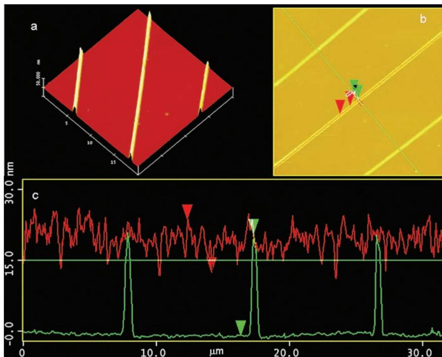
**Fig. 4.** Lines produced above the threshold for continuous line generation. (a) Topographic image in tapping mode. (b) Z projection of these three lines and (c) Cross-section (green) and longitudinal view (red) of the three lines. The width remains always about 500 nm, given by the focal spot size, and the height is 20 nm. The laser power was 3 mW and the scanning speed  $100 \mu\text{m s}^{-1}$
