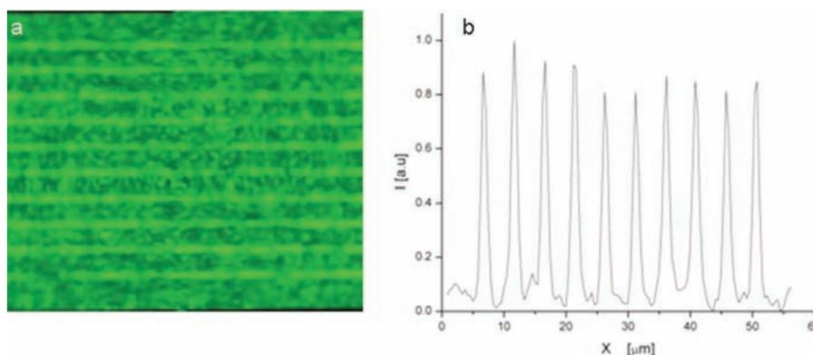
**Fig. 5.** Confocal image of nanofabricated 20-nm-high lines on a cover slip. (a) Projection of seven images Z stack with optical section separated by  $0.1 \mu\text{m}$ . (b) Average fluorescence cross-section.
