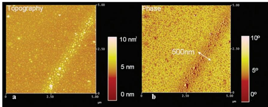
**Fig. 2.** AFM images of lines produced close to the surface polymerization threshold, where can be seen that the polymer growth starts on the surfaces of the substrate. The laser power was 1.5 mW and the scanning speed  $100 \mu\text{m s}^{-1}$ . (a) Topography and (b) phase image.
